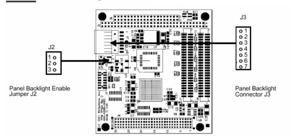
The Panel backlight enable jumper is located at J2. J2 must be jumpered 1-2 for Sharp type panels, and 2-3 for NEC type panels. An example jumpering for NEC type panels is shown below.
