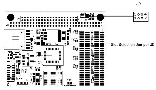
J9 is used to select the "slot" number of the PCI connection for the board. Each PC/104Plus board installed in a system must have a unique "slot" assignment and must not conflict with any PCI "slot" assignments on the CPU card. The jumperings for J5 are shown here :
