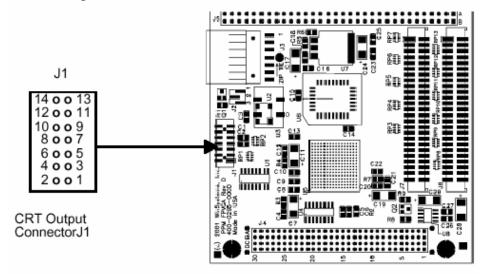
cable, part number CBL-234-1 is available from WinSystems to adapt J1 to a standard DB15 VGA connector. Pinout for J1 is shown here.
