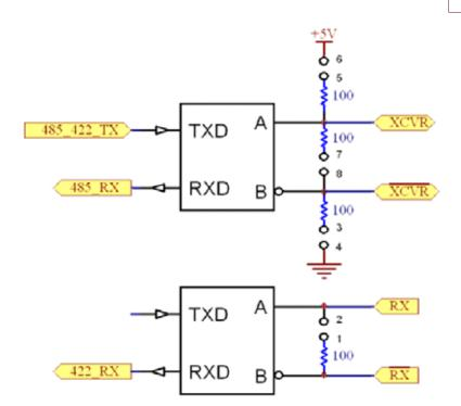
Note: Figure above illustrates the RS-422/RS-485 termination options installed when jumpers are installed on JP3, JP5, JP6, and JP10.
