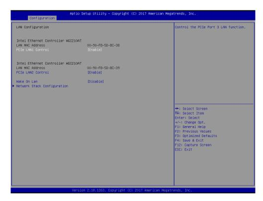
**PCIe LAN1 Control:** Control the PCIe Port 3 LAN function. Choices: Enabled (Default), Disabled
