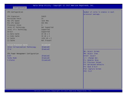
**Active Processor Cores:** The number of cores to enable in each processor package. Choices: Disabled (Default), Enabled
