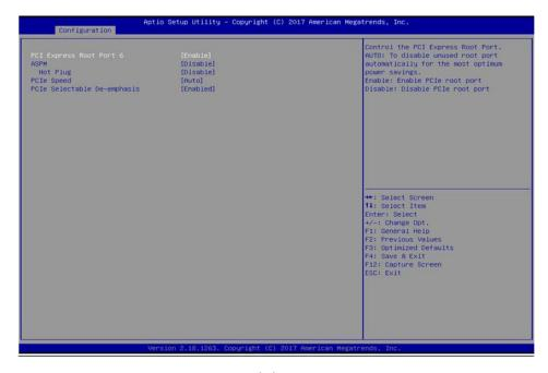
**PCI Express Root Port 6:** Control the PCI express root port. AUTO: To disable unused root port automatically for the most optimum power savings. Choices: Enable (Default, Enable PCIe Root port), Disable (Disable PCIe root port)
