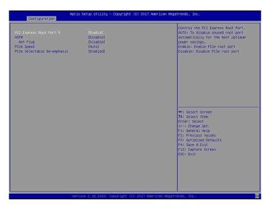
**PCI Express Root Port 5:** Controls the PCI express root port. AUTO: To disable unused root port automatically for the most optimum power savings. Choices: Enable (Default, Enable PCIe Root port), Disable (Disable PCIe root port)
