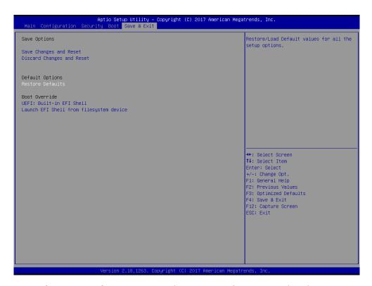
**Save Changes and Reset:** Reset the system after saving the changes.
