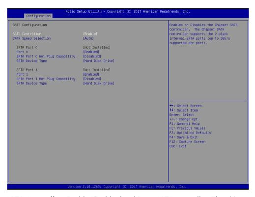
**SATA Controller:** Enable/disable the chipset SATA controller. The chipset controller supports the two black internal SATA ports (up to 3 Gb/s supported per port). Choices: Enable (Default), Disable
