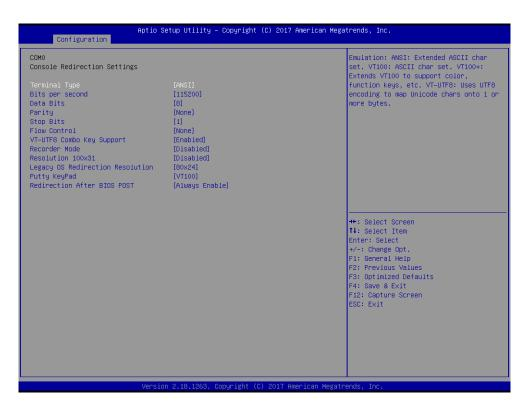
**Terminal Type Emulation:** ANSI: Extended ASCII char set. VT100: ASCII char set. VT100+: Extends VT100 to support color, function keys, etc. VT-UTF8: Uses UTF8 encoding to map Unicode chars onto 1 or more bytes. Choices: ANSI (Default), VT100, VT100+, VT-UTF8
