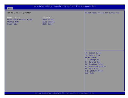
**Panel Profile:** Select panel profile for current use. Choices: 1280x1024 (Default), 640x480, 800x480, 800x600, 1024x768, 1280x800, 1280x1024,1366x768, 1440x900,1920x1080, OEM Profile
