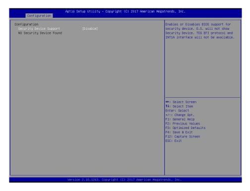
**Security Device Support:** Enable/disable BIOS support for security device. The OS does not show the security device. TCG EFI protocol and INT1A Interface is not available. Choices: Disabled (Default), Enabled
