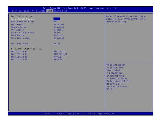
**Setup Prompt Timeout:** Set the number of seconds to wait for setup activation key. 65535 (0Xffff) means indefinite waiting. Choices: 2 (Default), 1-65535
