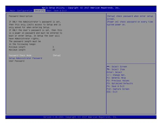
**Password Check Mode:** *Setup:* Check password when entering setup screen. *Power on:* Check password on every time system is powered on. Choices: Setup (Default), Power on
