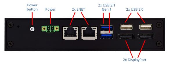
NOTE Configuration shown includes Power button module ADP-PS-433 and dual USB module ADP-USB-445.
