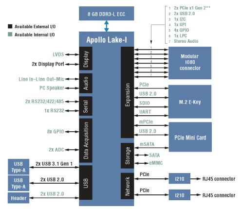
\*\*One PCle x1 lane is software switchable to 1x USB 3.1 Gen 1
