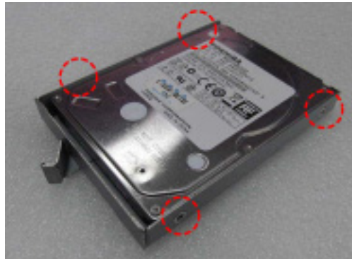
Figure 7-7: Secure HDD to tray
