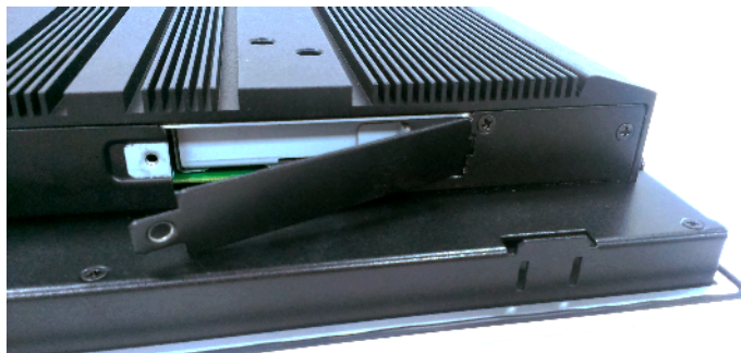
Figure 7-5: Remove HDD cover
