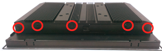
Figure 7-2: Securing the daughter board
