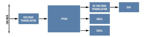
The PCM-MIO-A-1 utilizes a Lattice MachXO2 FPGA to communicate between the PC/104 ISA bus and the ADCs, DACs, and 48 DIO. The analog 16-bit inputs provide up to 100 Ksps, and ±25 V protection via the Linear Technology LTC1859 ADC converters. The DACs provide 12-bit outputs via the Linear Technology LTC2704.
