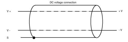
Thermocouple wires are color coded to indicate polarity. The positive thermocouple wire should be connected to the V+ terminal and the negative thermocouple wire should be connected to the V- terminal (the red thermocouple wire is negative by convention).
