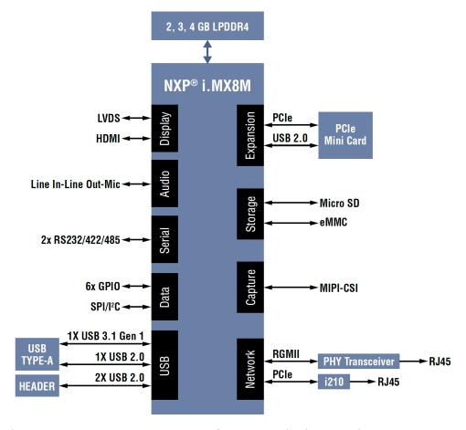
The WINSYSTEMS ITX-P-C444 SBC features a dual or quad-core processor and up to 4 GB of soldered down LPDDR4 RAM.
