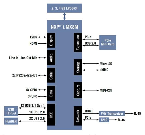
The WINSYSTEMS ITX-P-C444 SBC features a dual or quad-core processor and up to 4 GB of soldered down LPDDR4 RAM.
