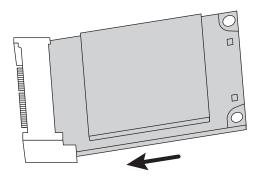
2. Push the free end of the card toward the circuit board, and then secure it with two 2 mm screws (WINSYSTEMS P/N G527-0000-400).
