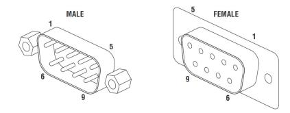
NOTE The following table contains standard pinouts of the EBC-C413 COM ports (COM1 through COM4) when connected to DB-9 connectors.
