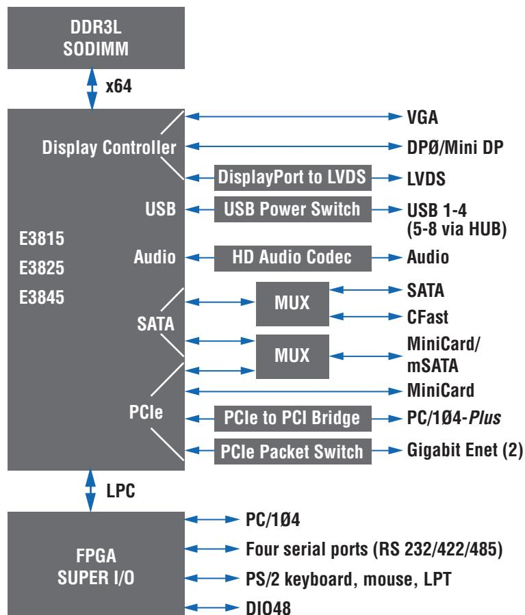
Three display interfaces (VGA, DP Mini DisplayPort, and LVDS) support dual video (up to two simultaneous independent displays) along with stereo audio. Communication interfaces include two Gigabit Ethernet ports, eight USB 2.0 ports with ESD suppression, four serial, 48 digital I/O lines with event sense, a watchdog timer, a PS/2 keyboard and mouse controller, and a parallel port (LPT).
