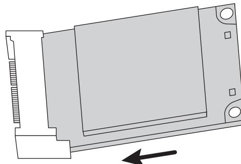
2. Push the free end of the card toward the circuit board, and then secure it with two 2 mm screws (WINSYSTEMS P/N: G527-0000-400).
