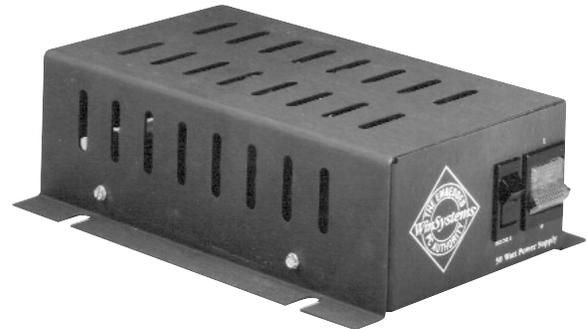
Operating temperature using convection cooling is from 0°C to +50°C with no derating. Its capacity is derated to 25W at 70°C. Forced air cooling will extend the operational temperature range.
