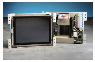
The Panel PC supports Linux and Windows XP, plus real-time kernels compatible with the x86 architecture.
