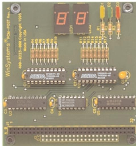
**Monitor LEDs** - Three LEDs on the PCM-POST provide a visual status of the power supplies. A red, green, and yellow LED is used for easy visual reference for the respective +5 volt, +12 volt and -12 volt supply lines.
