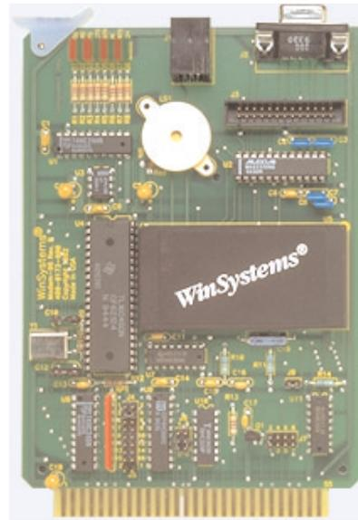
The Fax/Modem interface is a 16C550A compatible UART with a 16 byte Tx/Rx FIFO. It provides the parallel to serial interface between the bus and modem section. It will work with 7- or 8-bit characters and will handle 1 or 2 stop bits, even, odd or no parity, false start bit detection and automatic break detection.
